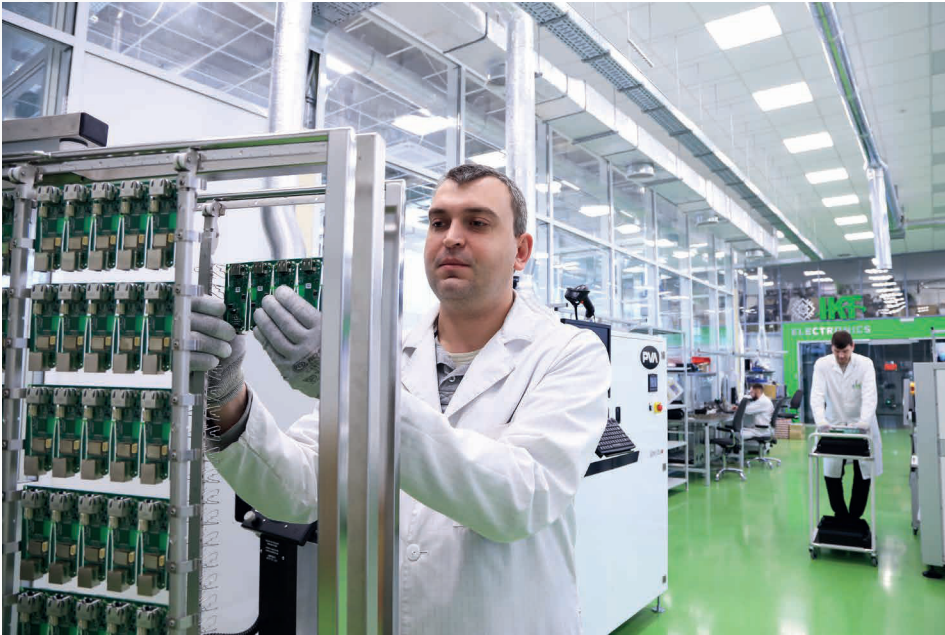
Automated system for cleaning printed circuit assemblies from flux residues SuperSWASH III
